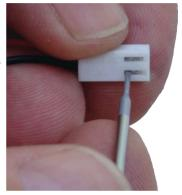
terminal. It must be raised slightly in order to regain it's locking function in the housing. This can be easily accomplished using the corner of a single-edged blade or X-Acto knife from the front or back of the terminal. Be careful not to bend it back up too far or it may break, this picture shows the maximum angle which you should bend it back.
